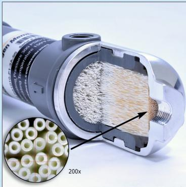
A typical membrane separator contains thousands of fibers that are bundled and encased at both ends in epoxy resin. The ends of the bundle are cut, which leaves the fiber bores open on both ends, allowing the gas to travel from one end to the other. The fiber bundle is enclosed in a suitable casing which protects the fibers and routes the gas properly.
